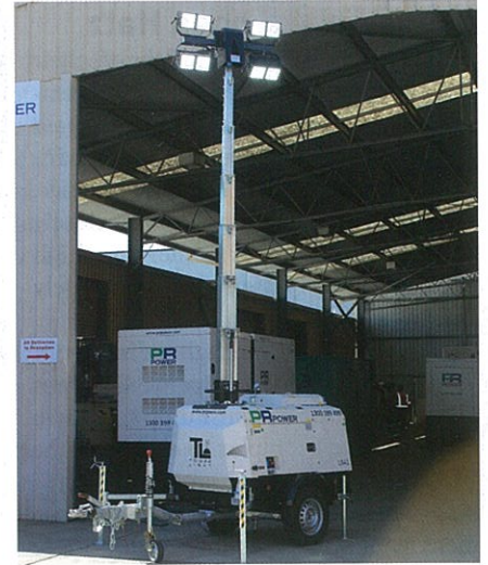
The PR-Hybrid-LED generates zero noise and carbon emissions while operating on battery power.
